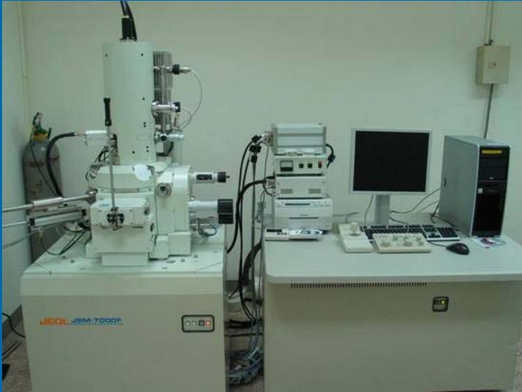
*Field-Emission Scanning Electron Microscope*
